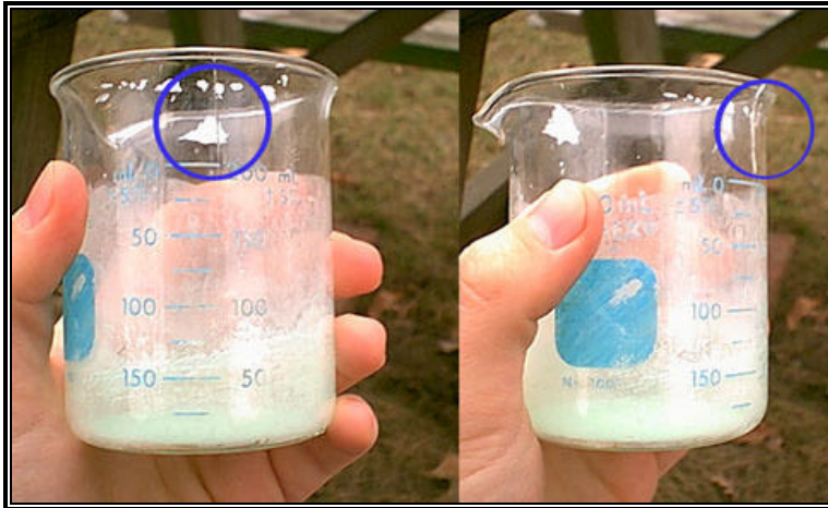
Cracks may be difficult to see when looking straight on at an object.
